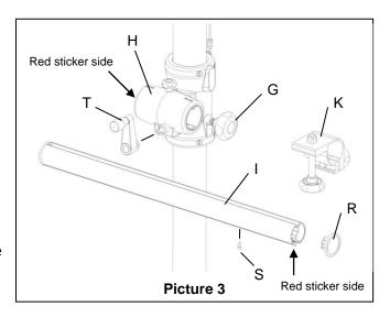
Place the recessed screw (S) back into the geared rack and remount the end-cap (R) to the cross arm. Slide the camera mount (K) onto the tube. The camera-mount can be moved across the tube and fixed secure in the wished position.
